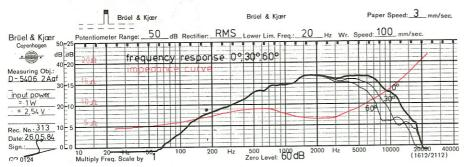
Significant flat impedance curve. Slope characteristics equal at 30° and 60° Easy filter design.
