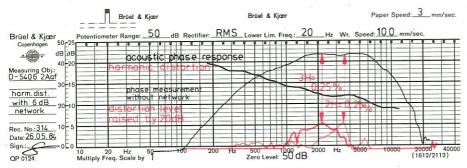
The acoustic phase proves the unproblematic handling of this midrange driver.
