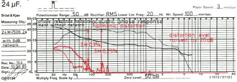
The harmonic distortions are at a very low level. At 100 Hz they are below 0.3%. At 50 Hz they do not reach 1%! Linear acoustic phase gives easy-to-handle 2-way system designs.
