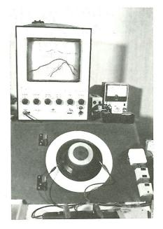
Despite most exacting production quality control there will always also remain human function. From voice coil to the complete driver the product will pass 8 to 12 quality control fields depending on type. Our demands for quality, for which DYNAUDIO is known, require exact observance of a low tolerance bandwidth. Tolerances of more than 0.0011 mm will cause rejection of the coil mandrel.
