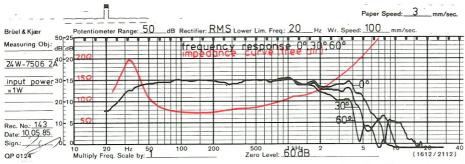
Curve is linear down to 40 Hz, only -3dB at 30 Hz. Smooth roll-off. Combined with D-28 the unit may be crossed at 2.5 KHz. Huge 3"/75mm voice coil gives impedance rise from 500 Hz easily to be compensated by 6.8 ohm and
