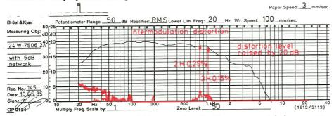
Using a fixed frequency of 100 Hz crossing it with a measuring frequency, the intermodulation is shown here.
