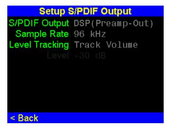
Set the S/PDIF Output from OFF to DSP. When the Preamp is set to 2-Ch Preamp mode the S/PDIF output on the back of the Preamp will represent the two-channel preamp output that is normally fed straight to channels 1-2 of the DAC in 2-Channel stereo Preamp mode. When you upload an Audioweaver design to the Preamp and force it into the Multi-Channel Preamplifier mode this will change from "Preamp-Out" to "Ch-9/10" indicating the additional two channels used in the 5-way crossover design.
