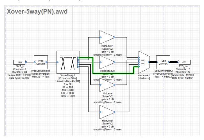
Note that the crossover block and interleave have 5 stereo pairs or 10 channels. We assign the lowest frequency band from the crossover block (top connection) to the additional stereo pair on the interleave (bottom connection) because this is the connection that represents channels 9/10 which are routed to the S/PDIF output.
