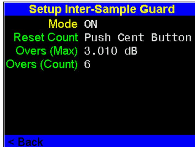
The guard calculated the worst case over to be about 3dB and applied this attenuation to the incoming samples to the SRC. As you can see in the scope shot below the signal is no longer distorted and the guard has done its job with minimal intervention !
