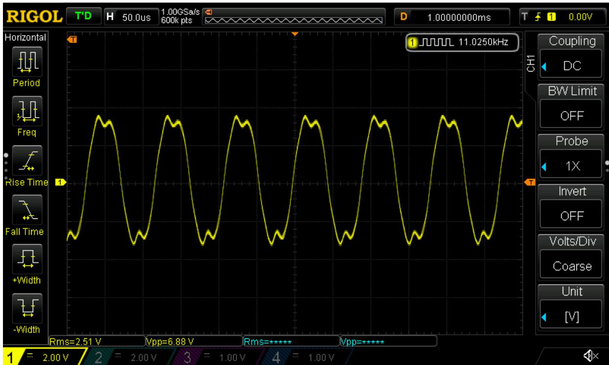
With the master volume set to -10dB we still get the same type of distortion which proves that the distortion is coming from the SRC and not the DAC !
