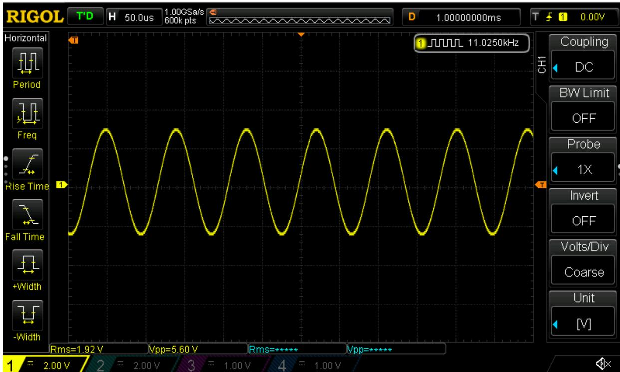
We can also achieve the same thing by turning on the Intersample Over Guard for the DAC which inserts a fixed 3.5dB attenuation on all 8 DAC channels. I.e from the main menu [Main Menu] → [Setup] → [Audio Setup] → [Intersample Guard] → [DAC = ON]
